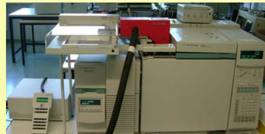
Fig. 1: TDS/GC/MS-system with Gerstel-autosampler (Mass Selective Detector, Agilent Technologies 6890N HP-SMS column 30 m x 250 \mu m x 0.25 \mu m)
